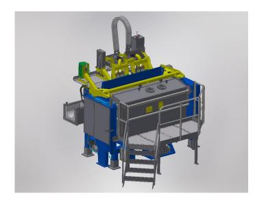
The DFF system is an inline Drain Free Filter system for mechanical filtration of liquid Aluminium. The Hycast DFF allows for high removal efficiency of inclusions compared to standard CFF systems by enabling the use of higher density filter plates. Reduced operating and remelt costs are possible due to complete draining of the filter box after operation. The unit utilizes standard dimensions of ceramic foam filter plates and can be supplied with single or double filter chamber.
