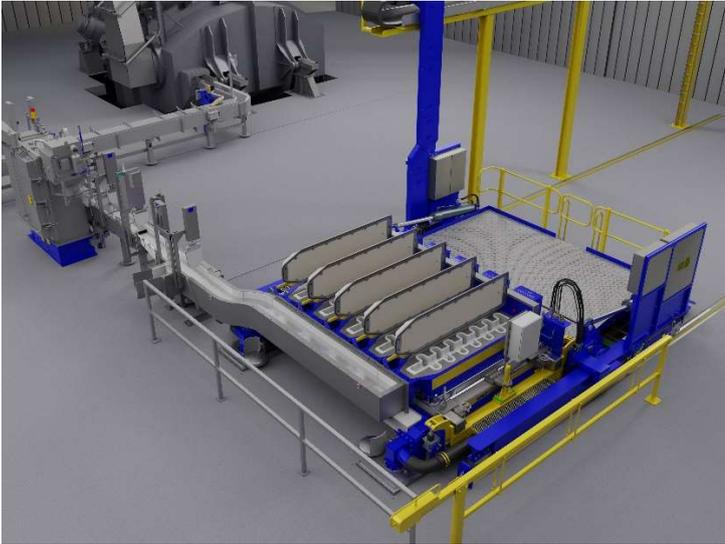
The Hycast® LPC (Low Pressure Casting) Billet Casting Technology is designed for the production of high quality extrusion billets with excellent surface quality and extrudability. Hycast® LPC gives you a billet with a unique and step change surface quality. Hycast® LPC Billet Casting Technology is ideal for production of larger diameters and hard alloys. Diameter range proven 90mm-520mm (3,5"-20,5"). Suitable for 1xxx, 2xxx, 3xxx, 4xxx, 5xxx, 6xxx, 7xxx and 8xxx alloys.
