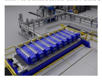
The Hycast® GC (Gas Cushion) Billet Casting Technology is ideal for production of high quality extrusion billets with excellent surface quality and extrudability. The system is proven worldwide over more than two decades in casthouses owned by Hydro Aluminium and its partners. Diameter range 120mm - 405mm (5" - 16"). Suitable for 1xxx, 3xxx, 4xxx, 5xxx, 6xxx and 8xxx alloys.
