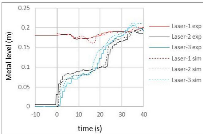
Figure 3. Measured and predicted metal level during filling.
