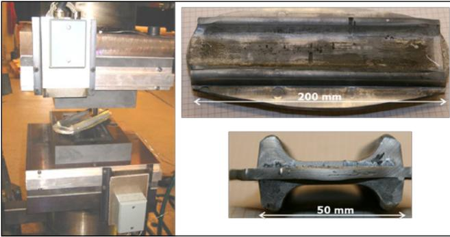
Figure 7. Forging die used on the laboratory-scale forging press (left) and detailed pictures of a forged piece (right).
