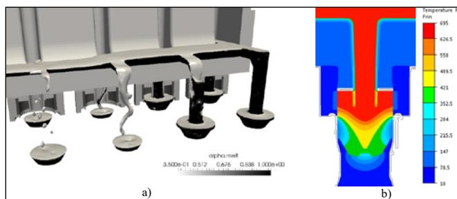
Figure 4. Detail view of predicted filling of the molds (a) and temperature distribution in LPC casting mold during start-up (b).
