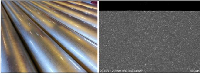
Figure 10. Billet surface and sub-surface structure of an AA7075 alloy cast with the LPC technology in 152 mm diameter.
