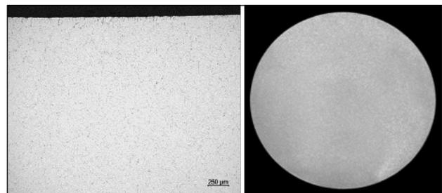
Figure 6. Micrograph of a typical surface region of the LPC 90 mm diameter cast forging ingots in alloy AA6082 (left). Macro grain structure of an as-cast AA6082 forging ingot (right).
