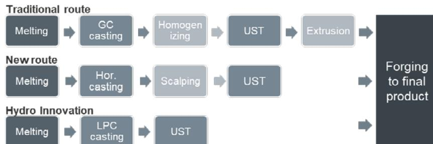
Figure 1. Alternatives for producing forging stock.
