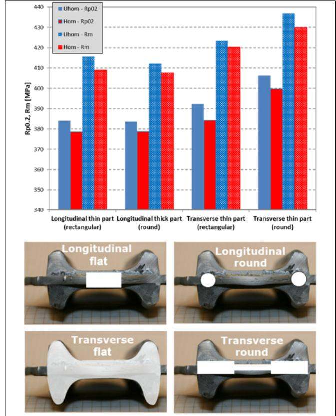
Figure 9. Tensile results from samples taken from different positions and directions of forged pieces. Results from unhomogenized material is represented by the blue bars and homogenized by the red bars.
