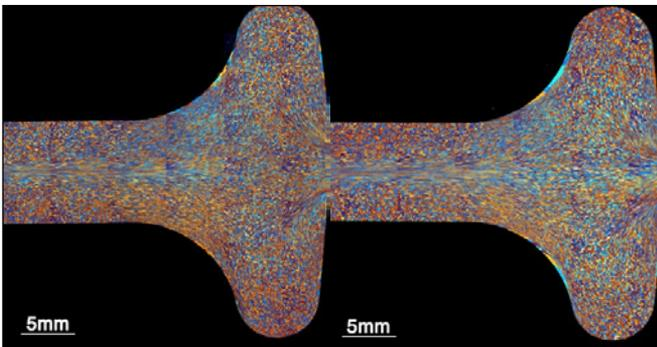
Figure 8. Light optical micrographs showing the grain structures in forged and solutionized samples (560°C/20 min). Unhomogenized material (left) and homogenized material (right).
