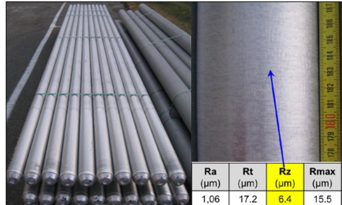
Figure 5. AA6082 cast forging ingots in 90 mm diameter (left) and a close-up of a typical surface with corresponding results from roughness measurements (right).
