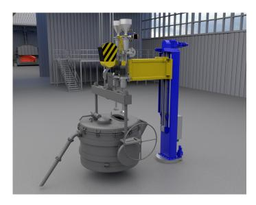
The Removal of alkaline metal is carried out by the introduction of aluminium fluoride (AIF3) to the liquid aluminium through a rotor using argon as transport medium. The Hycast® RAM system is a customized system that is tailor made for the tapping system on the smelter. Can be supplied with one or two-rotor solution.
