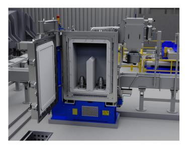
The Hycast® I-60 SIR sets the benchmark for the in-line refining of molten aluminium at casting centres. The unit has one reactor chamber with a baffle and two rotors, that can handle up to 70 t/hour.
