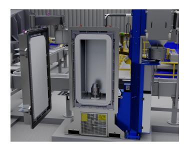
The Hycast® I-25 SIR is based on proven technology from the unique Hycast® I-60 SIR system including; inert atmosphere, drain free reactor, bottom mounted rotor and fully automated system. Dust filter system gives no dust emission to the environment. The unit has one reactor chamber and one rotor, that can handle up to 25 t/hour. Mobile preheating unit is included but pre-heating is normally not necessary between casts.
