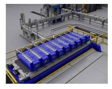
The Hycast<sup>®</sup> GC (Gas Cushion) Billet Casting Technology is ideal for production of high quality extrusion billets with excellent surface quality and extrudability. The system is proven worldwide over more than two decades in casthouses owned by Hydro Aluminium and its partners.
