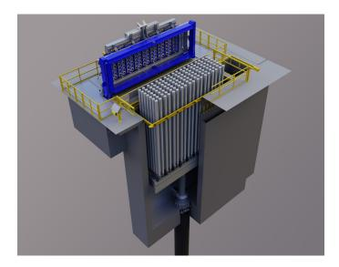
The Hycast<sup>®</sup> CMV comprises of a vertical casting machine with a single acting internally guided hydraulic casting cylinder. The mould carriage system is supplied as a tilt frame on a fixed foundation, or a rollaway mould carriage system with or without an integrated tilt-frame
